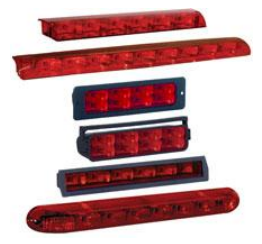
Our Module totally "Lights Up" when viewed within the 10° Left/Right, 10° Up/5° Down "Test Pattern", and therefore, has an EPLLA of ~6 x 1.5" = .9 in² each , where only Five meet the 4.5in², EPLLA requirement for FMVSS #108. We use at least 6 in all our new Modularized Designs
